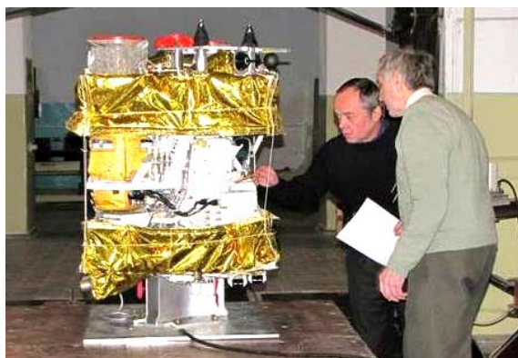
Fig. 8. Determination of the magnetic characteristics of the flying sample of the spacecraft «Sich-2» at the magnetometric stand of the Institute of Technical Problems of Magnetism of the National Academy of Sciences of Ukraine (Kharkiv, 2010)
