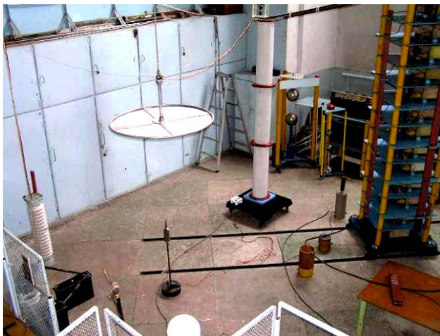
Fig. 9. General view of the high-voltage test stand of the R&DPCI «Molniya» of the NTU «KhPI», intended for testing lightning protection equipment of technical objects with commutation aperiodic voltage pulse with amplitude up to \pm 1 MV of time shape 250 \mu\text{s}/5000 \mu\text{s} and containing in the scheme a mobile superhigh voltage capacitor voltage divider of the type CDV-1, 2 [16]
