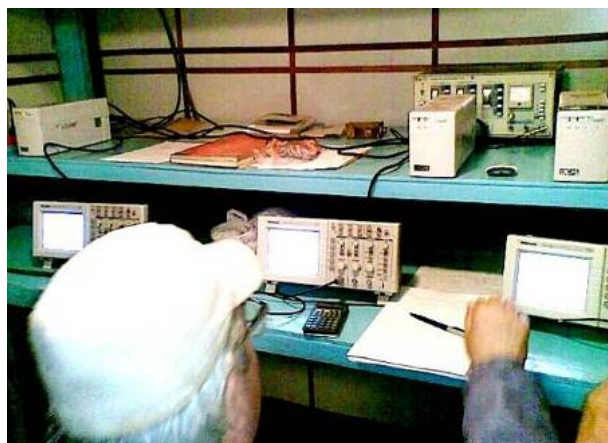
Fig. 5. External view of the placement of three Tektronix TDS 1012 digital storage oscilloscopes that register in parallel useful electrical signals from one SC-300M1 measuring shunt in a buried screened measuring hopper designed for metrology support of field testing of various technical objects for lightning resistibility [9]
